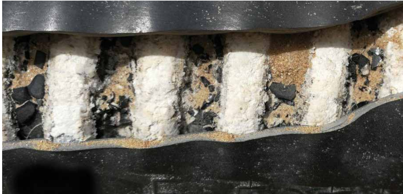
Corroded aluminium sheathed cable from the Middle East
