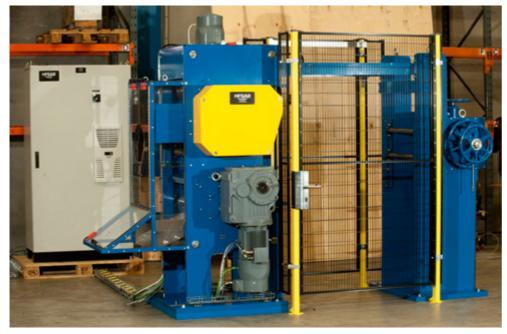
The CRRS cable stripping machine is designed for cables with up to 180 mm diameter. It removes defective insulation layers without damaging the subsequent layer below.
